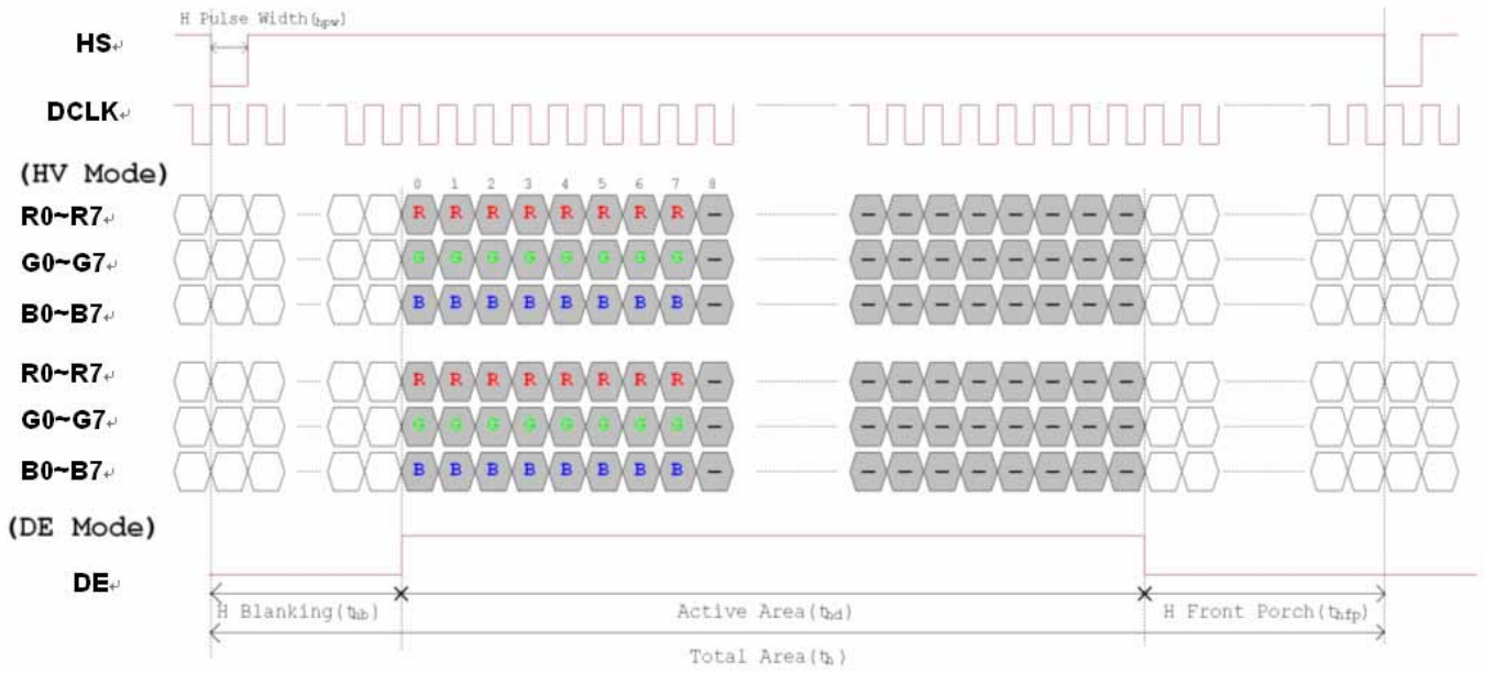
Figure 3. 1 Horizontal input timing diagram.
